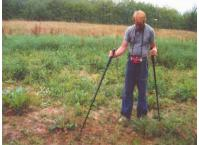
In order to determine various characteristics about a fault, such as severity, shape, corrosion behaviour, etc, various electrical measurements around the epicentre and from epicentre to earth are made for interpretation.
